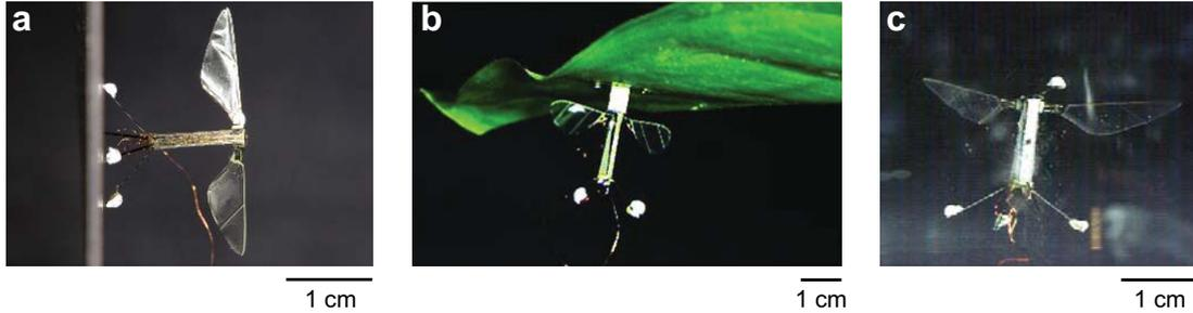
Figure 1.3: Novel RoboBee demonstrations. (a) A RoboBee perches on vertical surface through reinforcement learning. (b) A RoboBee sticks to a natural leaf through electrostatic adhesion. (c) A RoboBee swims in water. The functionalities demonstrated in (a), (b), and (c) are difficult to achieve in fixed wing aerial vehicles.
